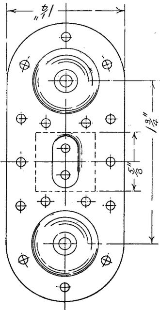
FIG. 38.—PLAN OF TOP CYLINDER COVER.
