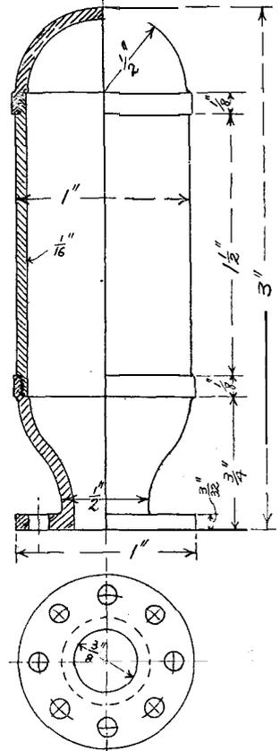
FIG. 47.--AIR VESSEL. (Full size.)
