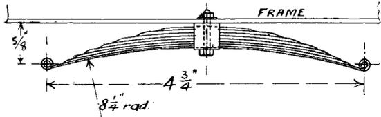
FIG. S.—TRANSVERSE SPRING. (Half full size.)
