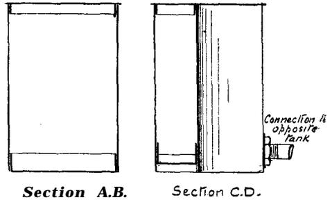
Note! The top of right-hand water tank is to be made in the form of a lid to facilitate removal of pump.
