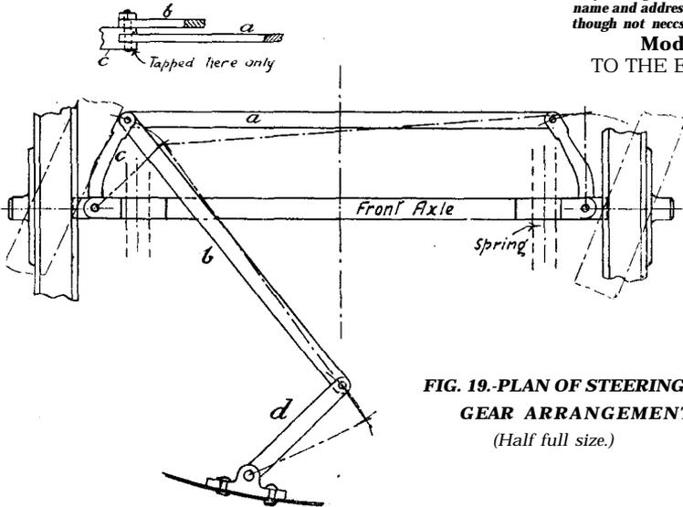
FIG. 19.-PLAN OF STEERING GEAR ARRANGEMENT. (Half full size.)
