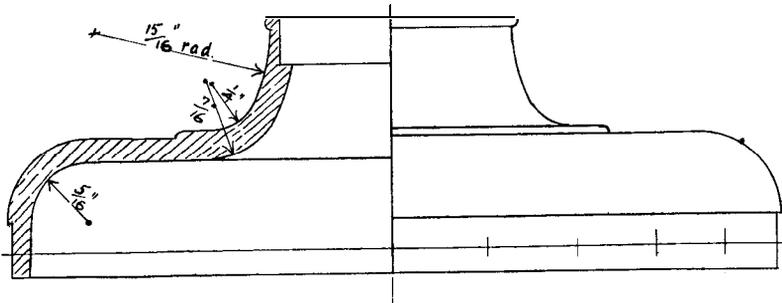
FIG. 24.-BOILER DOME. (Full size.)
