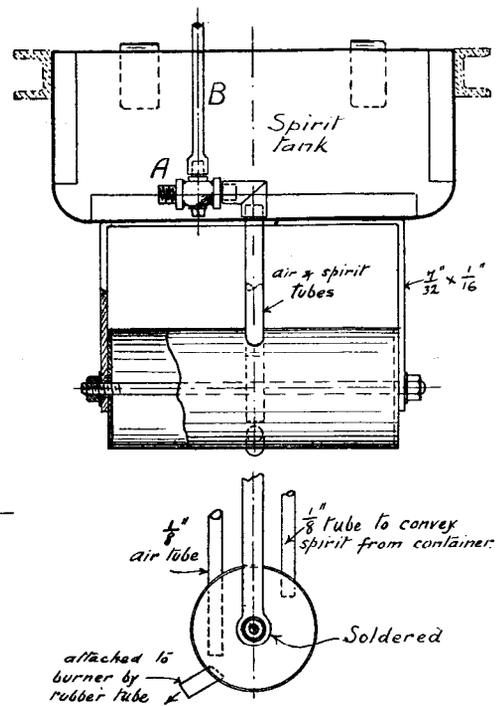
Fig. 32.--ARRANGEMENT OF SPIRIT RESERVOIR AND SUPPLY, SHOWING METHOD OF SUSPENSION BETWEEN THE FRAMES.
