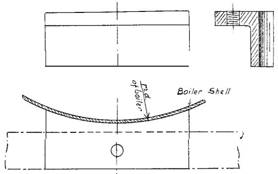
FIG. 27.-CASTING TO SECURE THE BOILER TO THE MAIN FRAME.
