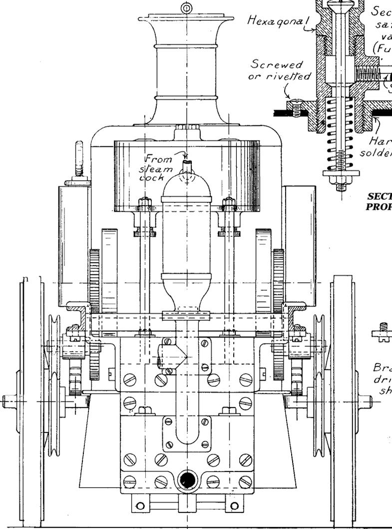
FIG. 42. SECTION THROUGH MODEL, SHOWING ARRANGEMENT OF ENGINE, PUMPS, AND GEARING.
