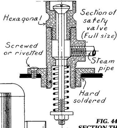
FIG. 44. SECTION THROUGH PROPOSED SAFETY VALVE.
