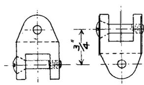
FIG. 5.—Two THUS FOR COUPLING FORWARD SPRINGS TO THE TRANSVERSE SPRING. (Full size.)
