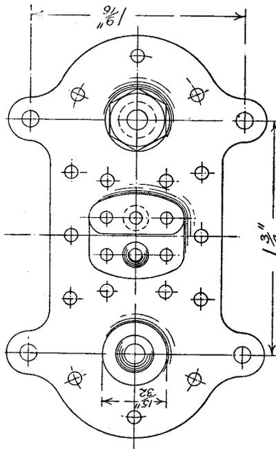
FIG. 39.—PLAN OF BOTTOM CYLINDER COVER.
