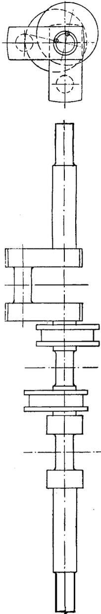
FIG. 41. DETAIL OF CRANKSHAFT. (Full SIZE.)
