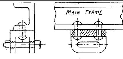
FIG. 3.—Two THUS FOR FORWARD ENDS OF REAR SPRINGS. (Full size.)
