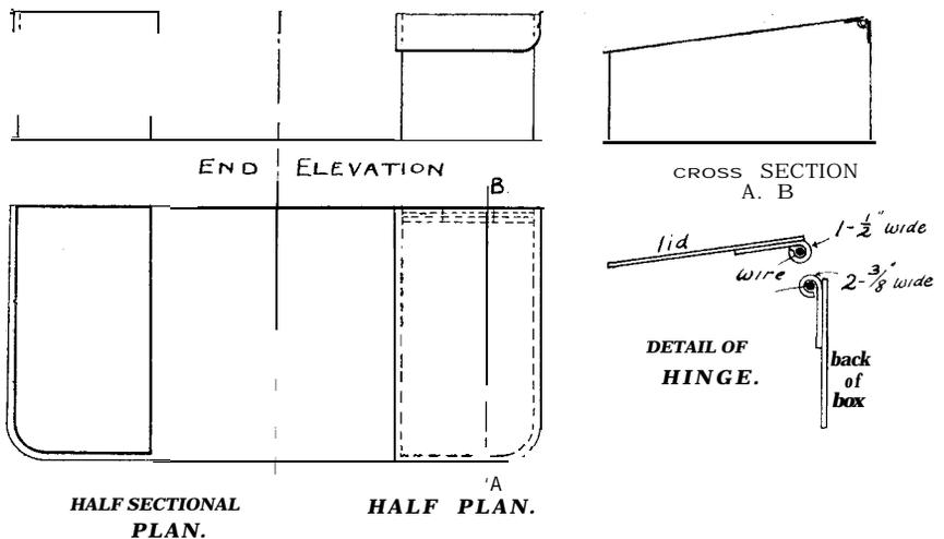
FIG. 29.-ENGINEER'S PLATFORM AND TOOL-BOXES. (Half full size.)
