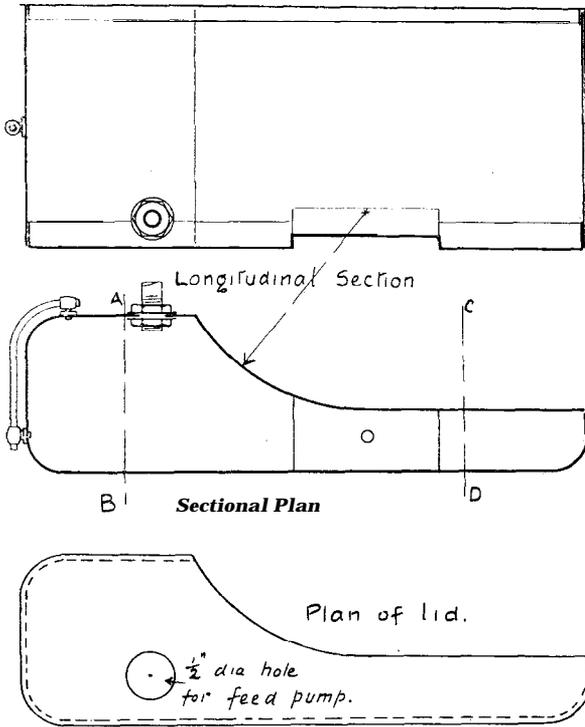
**FIG. 30.-DETAILS OF FEED-WATER TANKS.**
