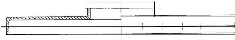
FIG. 25.-CIRCULAR PLATE TO FORM SMOKEBOX. (Full size.)
